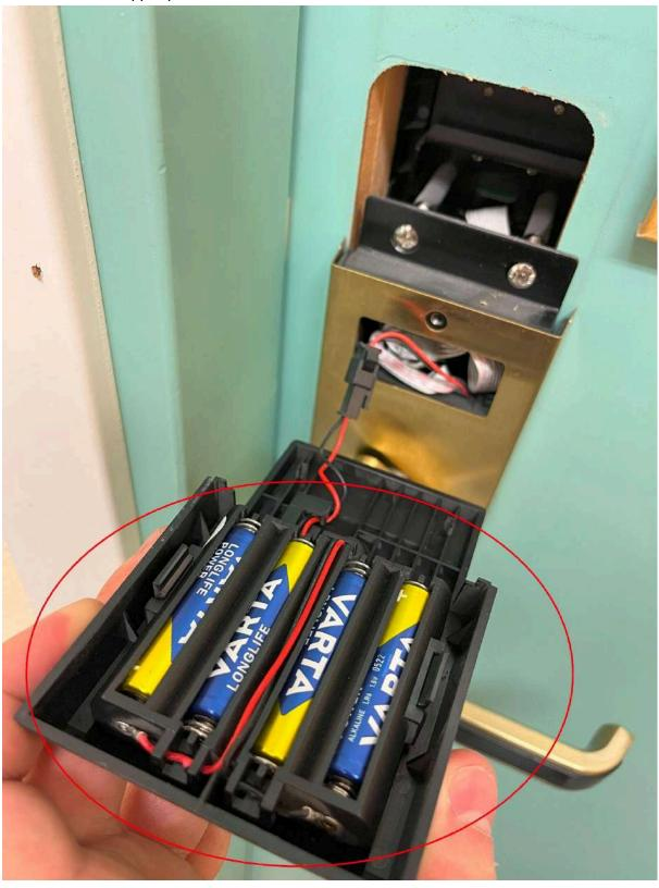
4. Disconnect the battery shell from the upper cover.
